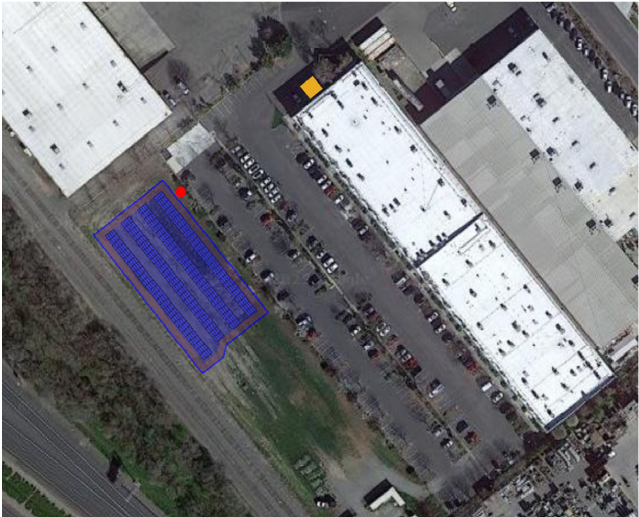
Santa Anita Court (Main Office) Building – (4) EV chargers (orange), (1) Pull box (red) and conduit to main switchgear
